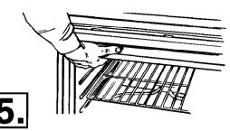
Remove and discard shipping base. Lift oven up into cabinet cutout using the oven opening as an area to grip.
